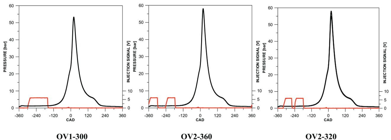
Fig. 2. Injection signal and pressure traces averaged on 400 consecutive cycles for the selected operating conditions
