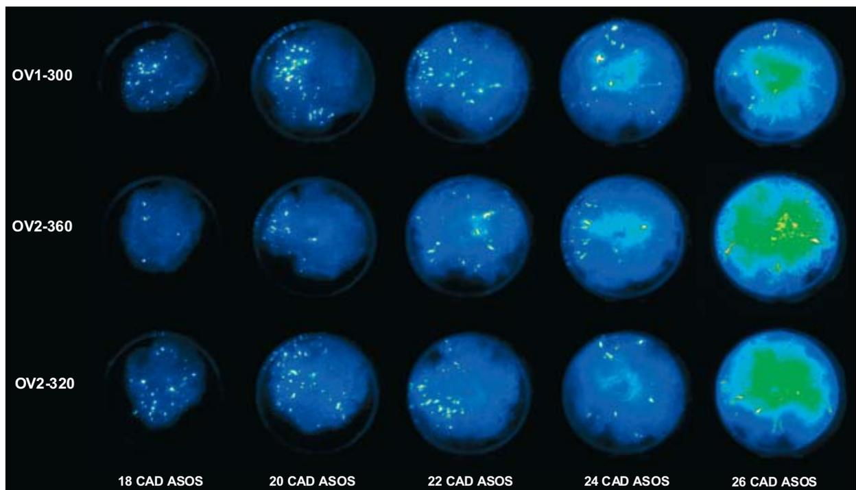
*Fig. 4. UV-visible flame emission detected in the combustion chamber for the selected operating conditions*
