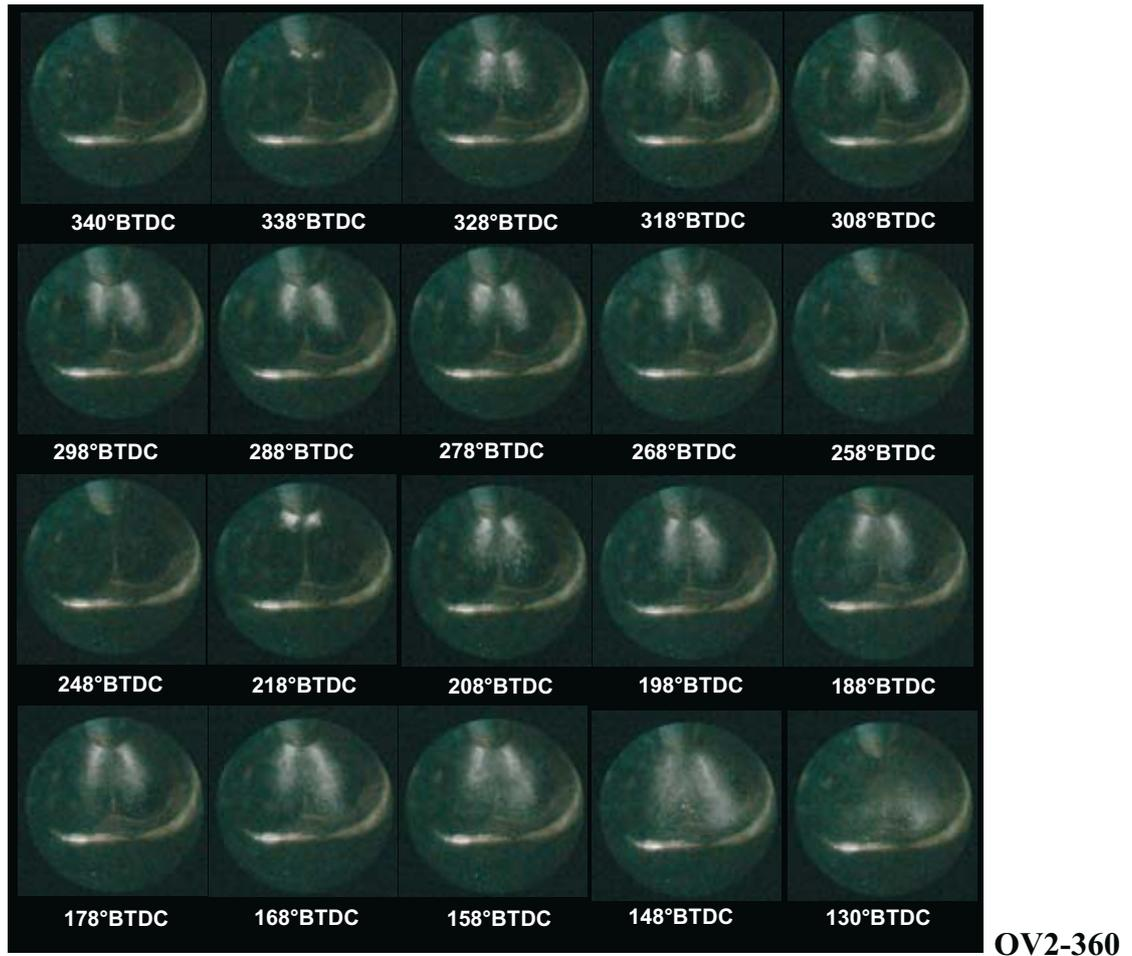
*Fig. 3. Fuel injection detected in the intake manifold for the conditions OV1-300 and OV2-360*
