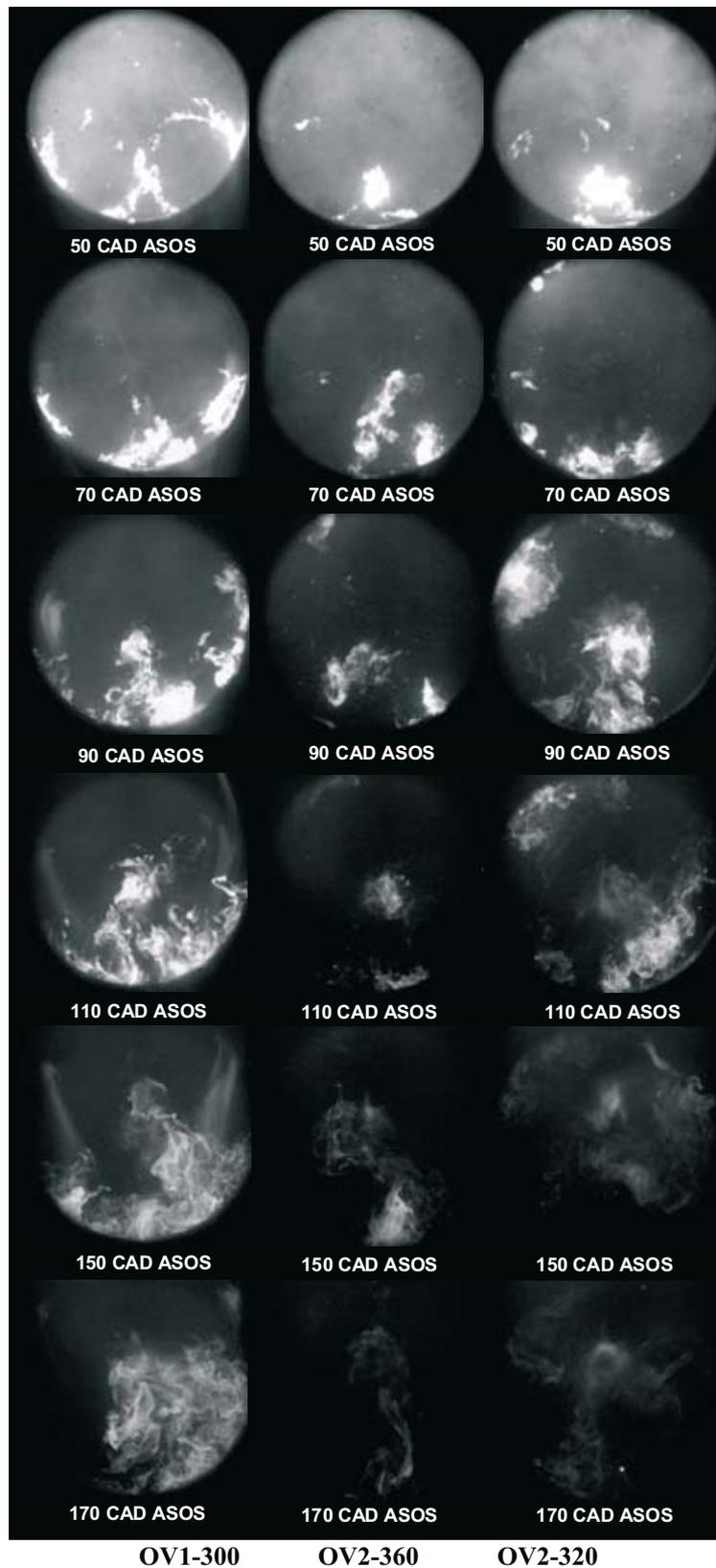
*Fig. 6. Flame emission detected in the late combustion phase*
