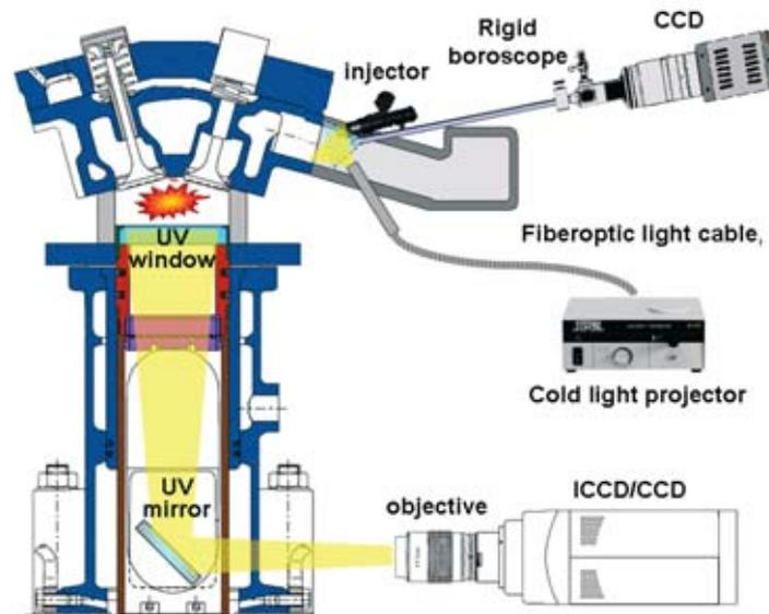
Fig. 1. Sketch of the experimental apparatus the optical investigations
