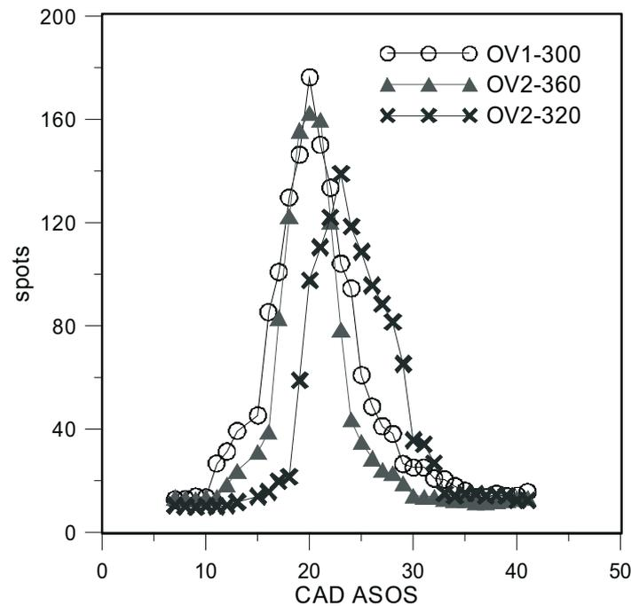
Fig. 5. Number of the bright spots detected in the combustion chamber for the selected operating conditions
